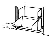
Hold side-lock latch and tilt side of drawer until the latch clears the drawer front.
